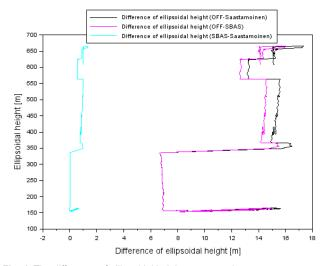
Fig. 4. The difference of ellipsoidal height at approach to landing procedure
