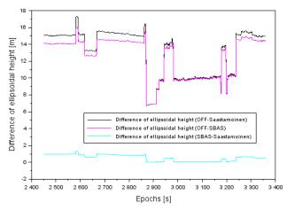
Fig. 3. The difference of ellipsoidal height at approach to landing procedure
