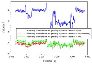
Fig. 5. The accuracy of ellipsoidal height at approach to landing procedure
