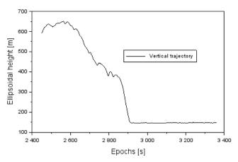
Fig. 1. The vertical trajectory at approach to landing procedure
