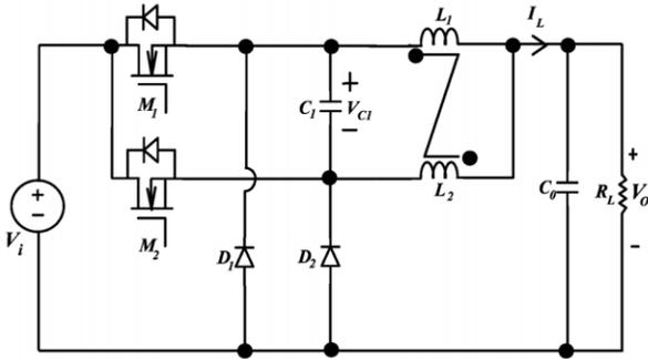
Fig. 4. IBC with a single-capacitor snubber [9].
