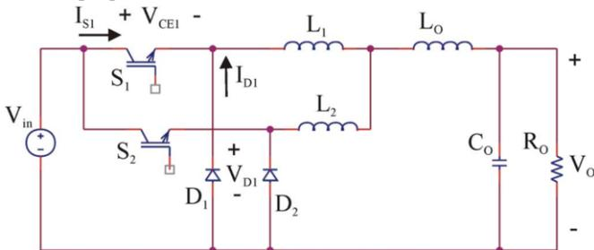
Fig. 7. Interleaved zero-current-transition (ZCT) buck converter [12].
