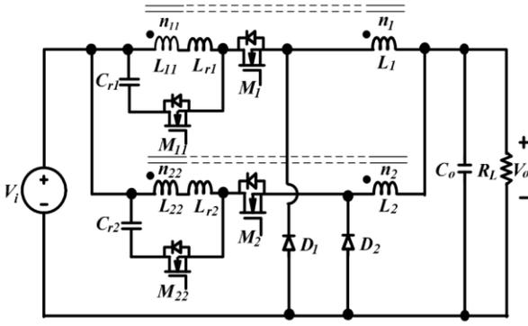
Fig. 10. Interleaved coupled-buck converter with active-clamp circuits [15].
