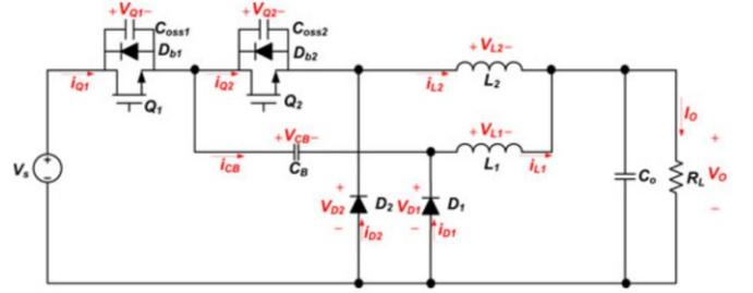
Fig. 11. IBC with extended duty cycle [16].
