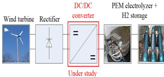
Fig. 2. Hydrogen generation pathways from wind turbines.
