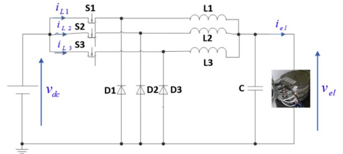
Fig. 3. IBC connected with the electrolyzer.
