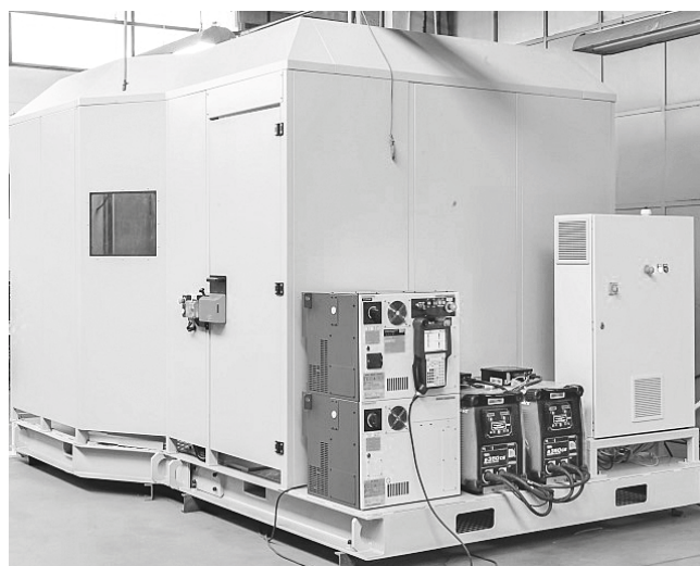
Rys. 3. Kabina spawalnicza stanowiska Plug and Produce Fig. 3. Welding Cabin Plug and Produce
