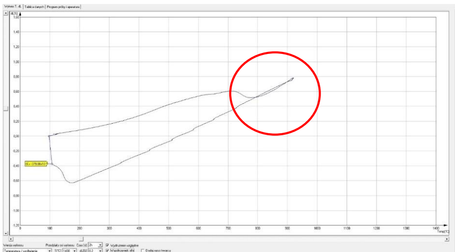
Fig. 8. Dilatometric curve chart for the 1.2709 MARAGING grade steel. The vertical axis shows the relative dimensional changes of the sample ranging from 0-1,6 [%]. Temperature range on the horizontal axis 0-1400 °C
