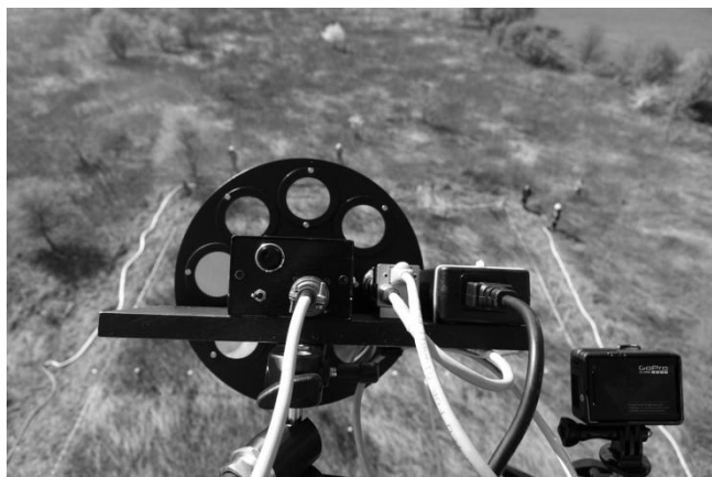
Fig. 5. Camera installed in the platform together with an automatic filter changer
