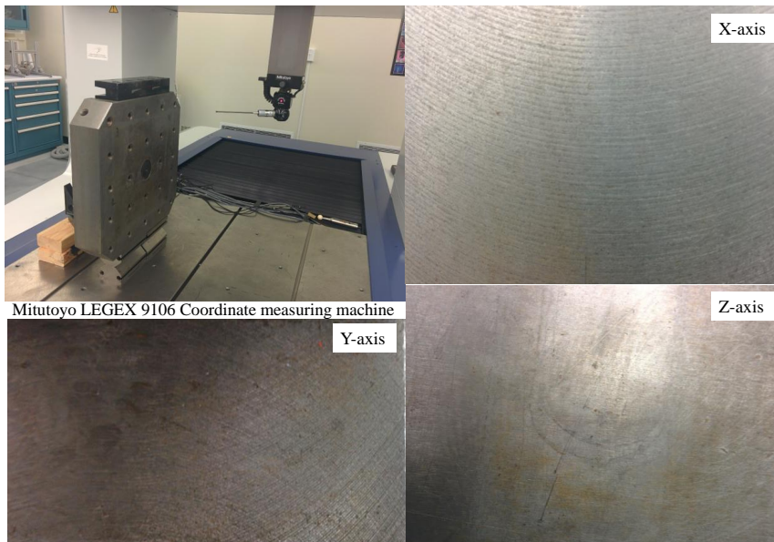
Fig. 8. The Coordinate Measuring Machine (CMM) and surface quality at X-, Y- and Z-direction
