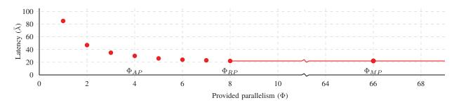
Fig. 6. Latency versus parallelism plot for an 8-point IDCT function with average parallelism ( $\Phi_{AP}$ ), required parallelism for its ASAP latency ( $\Phi_{RP}$ ), and maximum parallelism ( $\Phi_{MP}$ ) marked
