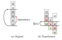
Fig. 8. Simplified schedules for the original (listing 2) and transformed (listing 3) version of a loop showing an inter-iteration dependency. The original schedule shows the inter-iteration dependency which constrains software pipelining. The transformed schedule has been software pipelined and assumes that A and B are stored in different memories.
