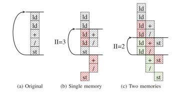
Fig. 7. Simplified schedules of the loop shown in listing 1 showing the original sequential schedule and two software pipelined versions demonstrating the influence of different memory mappings. Operations from different loop iterations are distinguished by their background color and texture. Only the kernel operations are shown in these schedules, address calculation and control-flow operations are hidden for brevity.
