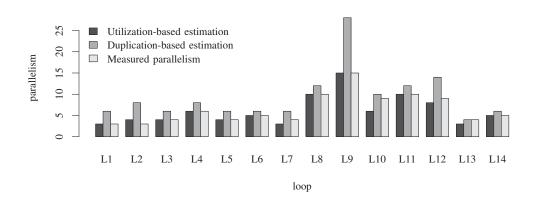
Fig. 9. Comparison of estimated parallelism versus observed parallelism after software pipelining in custom built architectures.
