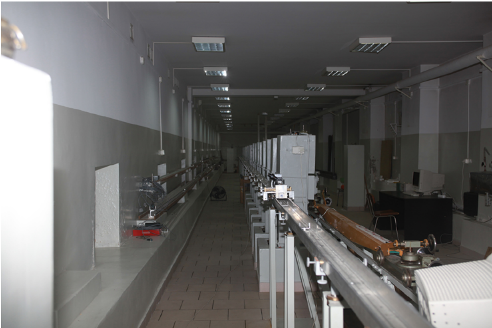
Fig. 1. Optical baseline in Geodetic Metrological Laboratory
