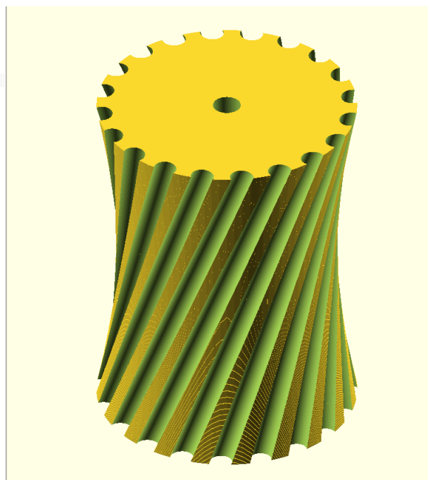
Fig. 32.3 One-sheeted hyperboloid as gear from transmission between skew axes
