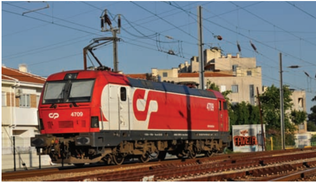
Fig. 4. LE 4709 locomotive (1668 mm, 25 kV 50 Hz) at Valongo (Estação) station, Portugal (21 June 2010) [photo by T. Miranda / Wikimedia Commons]
