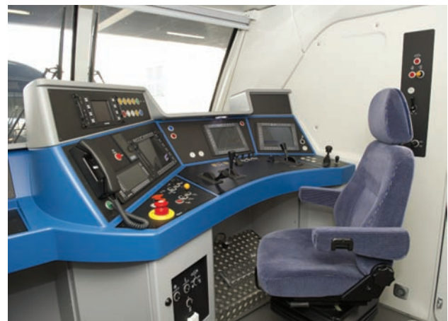
Fig. 11. Control panel of the Vectron locomotive [photo by Siemens]
