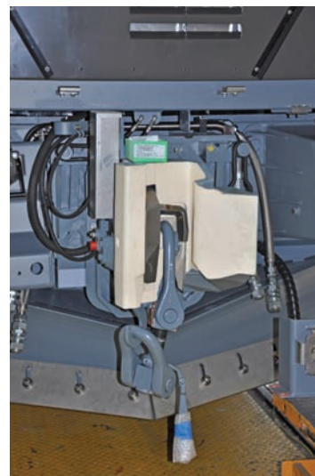
Fig. 24. LAF (UIC + SA-3) mixed coupler on VR's Vectron locomotive [photo by M. Graff]
