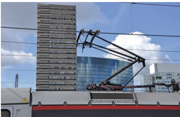
Fig. 19. The pantograph of an SNCB-owned HL 1800 class locomotive [photo by M. Graff]
