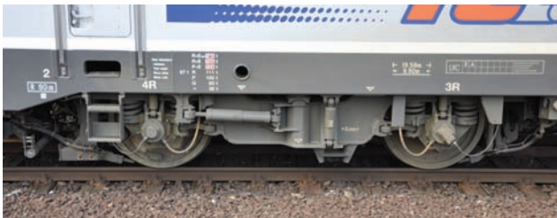
Fig. 17. The bogie of a PKP IC-owned EU44 series locomotive [photo by M. Graff]
