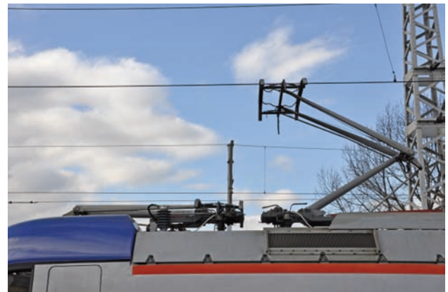
Fig. 20. The pantograph of a PKP IC-owned EU44 class locomotive [photo by M. Graff]
