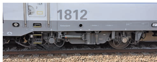
Fig. 15. The bogie of an SNCB-owned HL 1800 series locomotive [photo by M. Graff]
