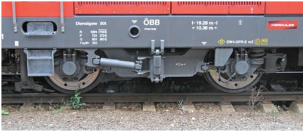
Fig. 16. The bogie of an ÖBB-owned ER20 series locomotive [photo by M. Graff]
