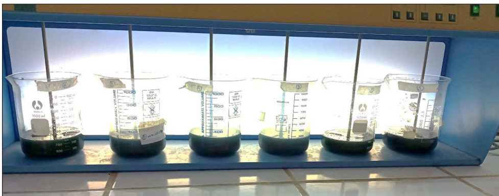
Figure 1. Jar test equipment for Coagulation-Flocculation experiment
