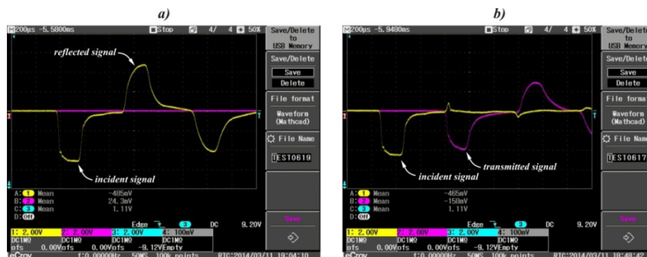
Fig. 4. The raw viscoelastic wave signals measured by the strain gages:
