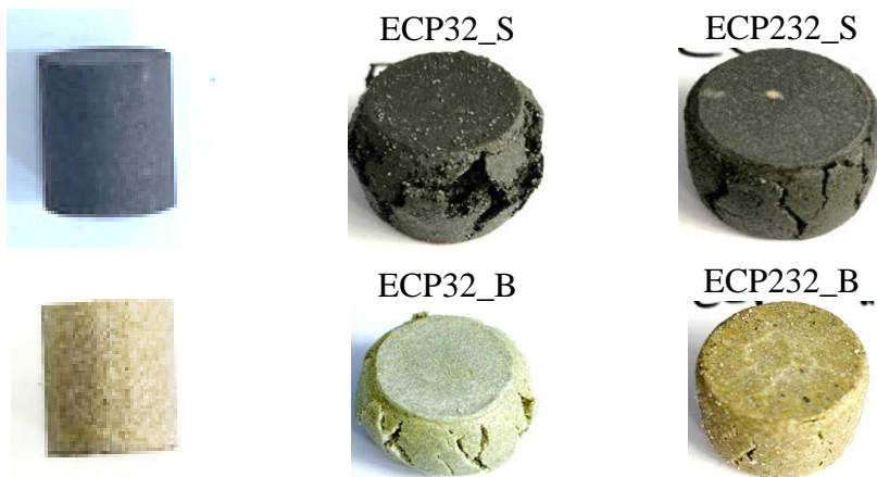
Fig. 3. The structural configuration of cylindrical composites after testing (left: specimens before compressive loading application; middle and right: specimens after compression testing)
