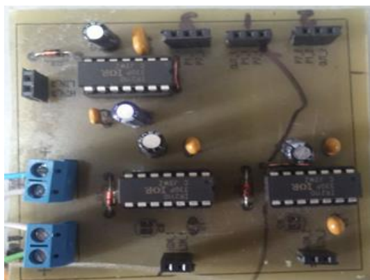
Fig. 27. The photo of the PCB board for the IR2110 driver circuit
