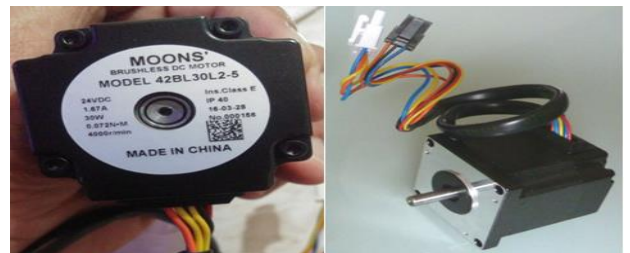
Fig. 3. The 42BL30L2-5 is a BLDC motor manufactured by MOONS' Company
