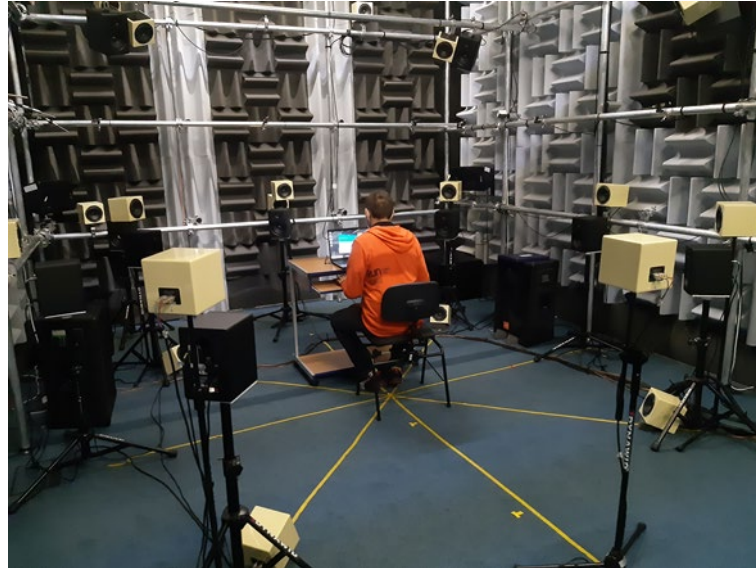
Figure 1. Laboratory facility for testing wind turbine noise annoyance.
