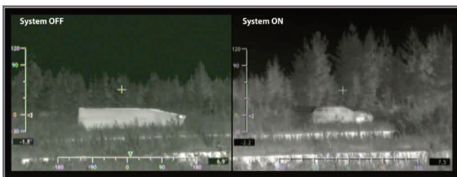
Fig. 7. Thermal masking method ADAPTIV from BAE Systems [8]
