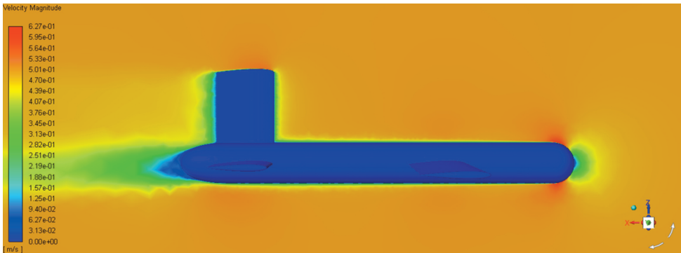
Figure 11. Velocity magnitude around the glider body, V=0.5 m/s, angle of attack = 0^\circ . X0Z geometry plane
