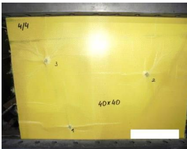
Photo 8. Composite after firing with rounds: 1) 357 Magnum bullet JSP, 2) 9x19 mm bullet FMJ, 3) 357 Magnum bullet FJCBSC
