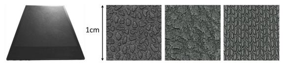
Figure 5. Example of test plate (21x15 cm) and microscopic view of texture 1 – 3 (from left to right)
