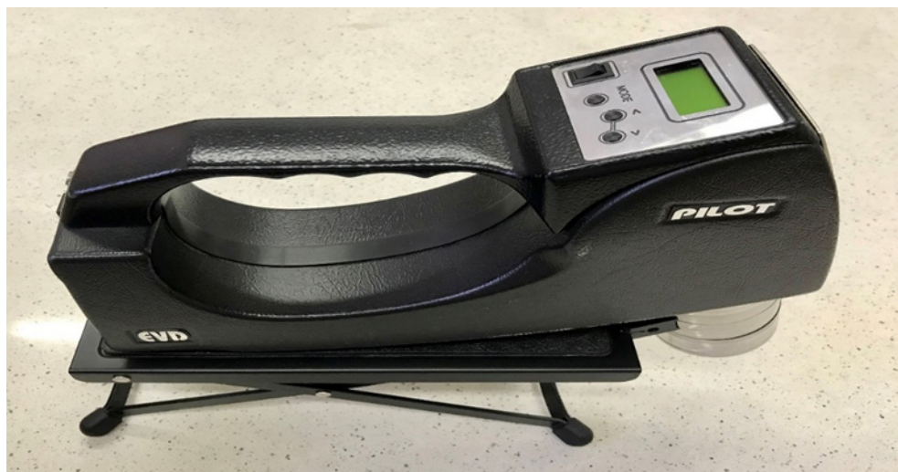
Figure 2. Detector PILOT-M with desorber
