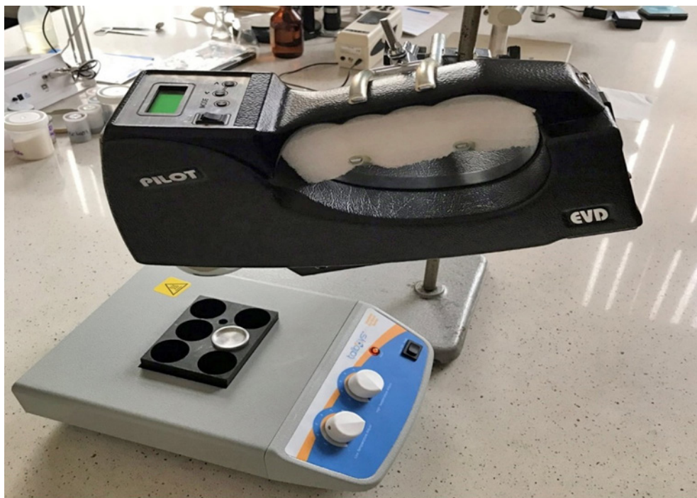
Figure 3. The experimental set-up applied for studying of the influence of temperature on explosives detection (in the lower part Talboys heater, in the upper detector PILOT-M)
