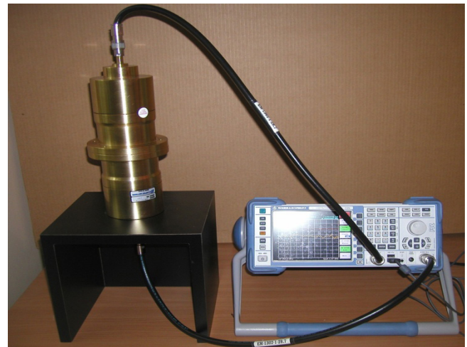
Figure 5. View of the measurement setup used for the determination of the EMI SE.
