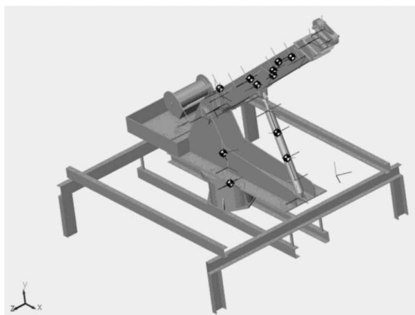
Fig. 4. Visualization of a sample SimMechanics model (model of laboratory truck crane)
