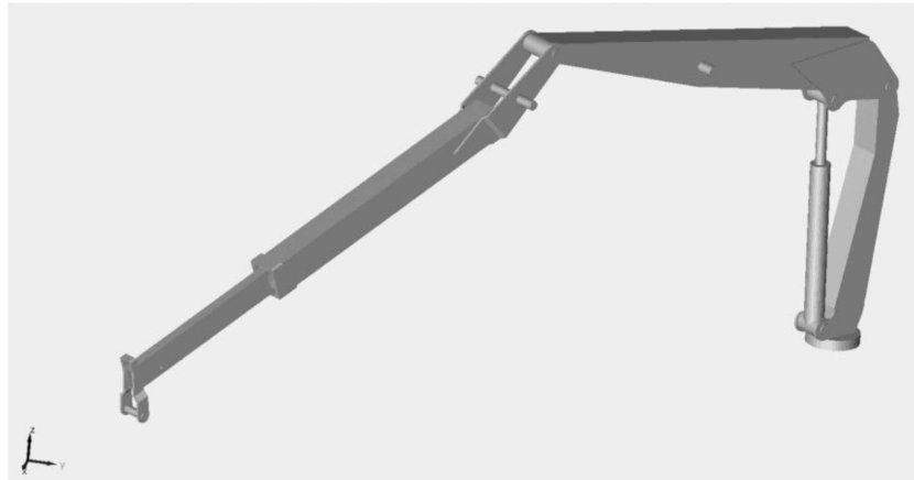
Fig. 13. Visualization of the forest crane SimMechanics model
