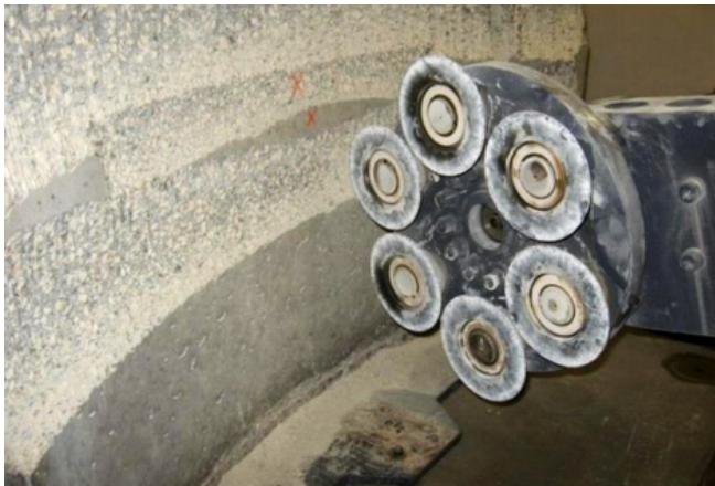
Fig. 13. A view of the cut after one of the mining tests in the horizontal plane
