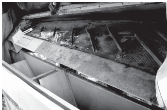
Figure 1 and 2. Separating deck of the FGX-1 air concentrating table [source: Photo by Wojciech Sobko]
