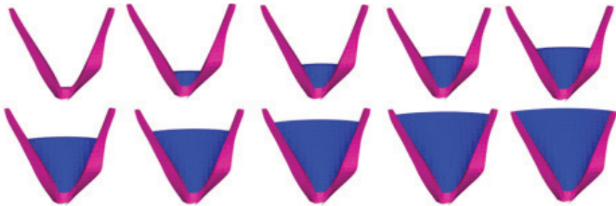
Fig. 8. Stage construction considered for static analyses.
