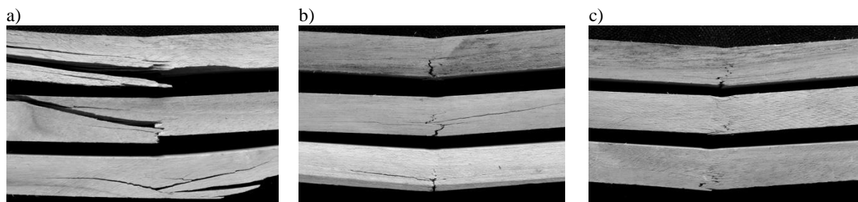
Figure 10. Typical damage pattern after MOE s -MOR tests (according to ASTM 143-94:2000): a) cross-grain tension, b) simple tension, c) brash tension
