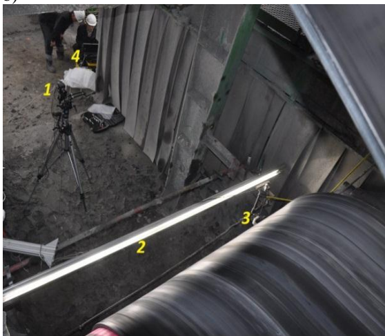
Fig. 8 Visual module during measurements on conveyor: a) view of LED illuminator, b) screen protecting against weather conditions
