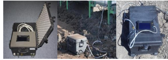
Fig. 3. View of open measuring system box with visible tablet and wiring and during its operation at belt conveyor
