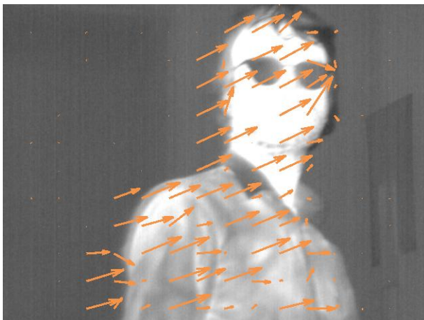
Fig. 2. Optical-Flow estimated from infrared image using Farneback method
