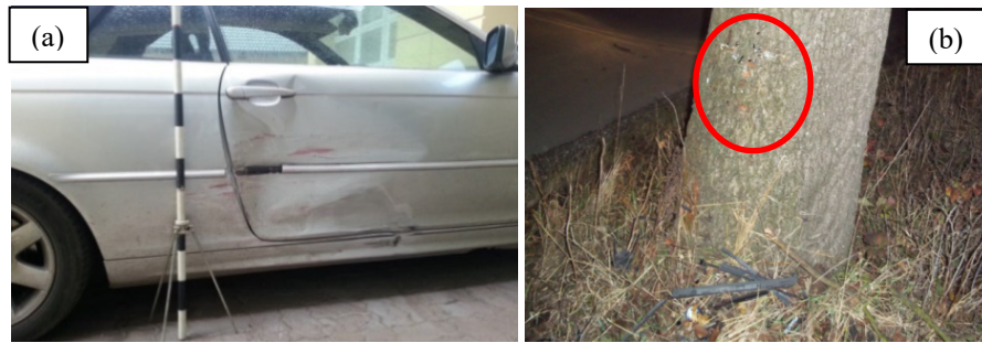
Fig. 4. Characteristic marks in the form of paint accumulation on a vehicle of the claimant (a) and pieces of paint impacted into a tree trunk - indicated obstacle (b)
