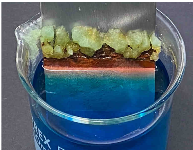
Fig. 16. Crystals of iron(II) sulphate, formed at the interface of mild steel reacting with copper sulphate solution
