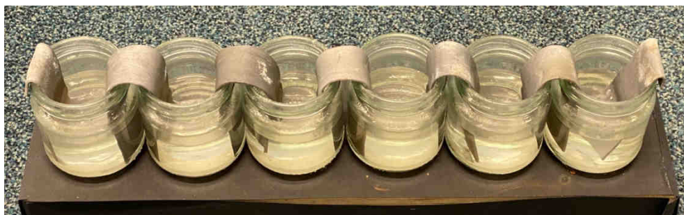
Fig. 12. Home-made lead/acid battery, suitable for teaching purposes
