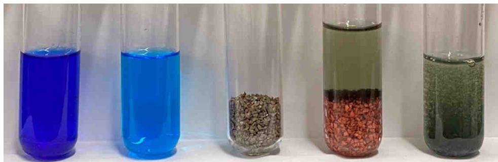
Fig. 15. The reaction of iron with copper sulphate solution - nos. 1-5 from left to right
