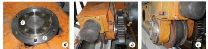
Fig. 6. Force transducer type HDT: a) components, b) HDT fitted in the driven wheel bearing housing - the cogwheel side; c) HDT fitted in the driven wheel bearing housing - the wall side
