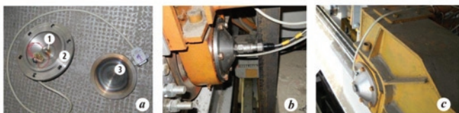
Fig. 5. Force transducer type CST: a) components; b) CST with a mounted accelerometer, fitted in the non-driven wheel bearing housing; c) CST fitted in the non-driven wheel bearing housing on the wall side
