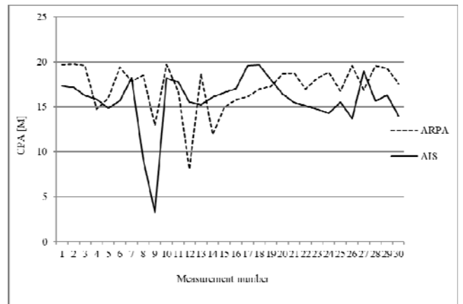
Figure 12. CPA values of the ship "Ocean Trader" (meeting situation 16) presented by ARPA and AIS [8]
