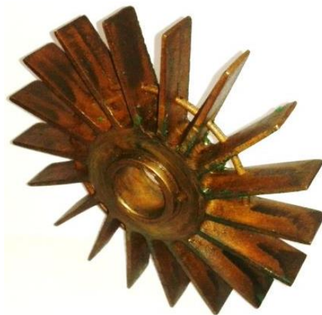
Fig. 3. The pump impeller used for modeling
