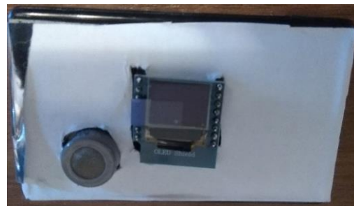
Fig. 24. CO and CO 2 module of the Smart Wagon system (author's picture)
