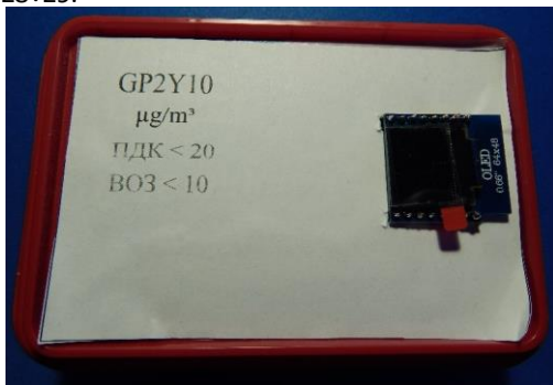
Fig. 28. Dust sensor module of the Smart Wagon system (author's picture)
