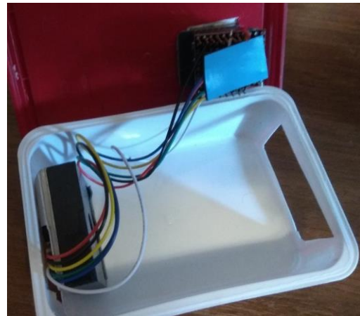
Fig. 29. Inside of dust sensor module of the Smart Wagon system (author's picture)
