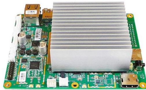
Fig. 6. System board of the Smart Wagon system developed by the author [5]
