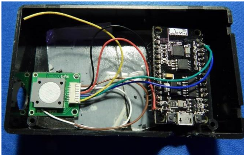
Fig. 17. Inside of formaldehyde sensor module of the Smart Wagon system (author's picture)
