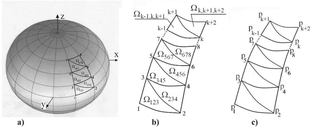
Fig. 8. Lubrication region  $\Omega_\Sigma$ : a) localization on the elliptical surface, b) region  $\Omega_\Sigma$  as a sum of elliptical triangles, c) measured pressure values in the vertexes of particular elliptical triangles
