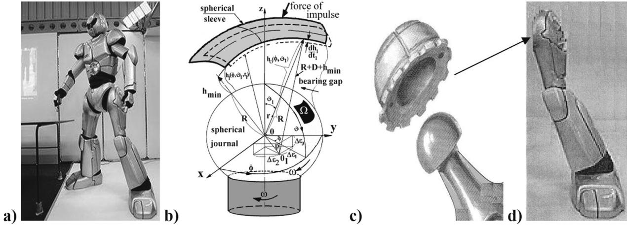
Fig. 1. Robot with spherical bearings: a) Illustration of the robot, b) spherical gap height and eccentricities, c) connection with the artificial sleeve in robot, d) the foot and leg of the humanoid robot
