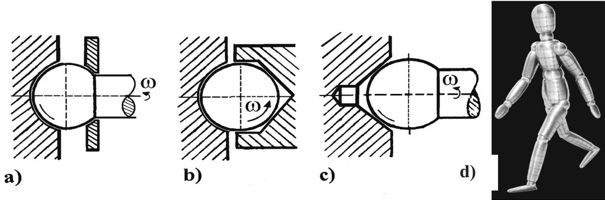
Fig. 3. Spherical and elliptical bearings: a) spherical journal together with a shaft and spherical sleeve, b) individual elliptical ball with conical sleeve, c) elliptical journal together with a shaft and conical sleeve, d) localization possibilities of the elliptical slide bearing between movable limbs occurring in humanoid robots
