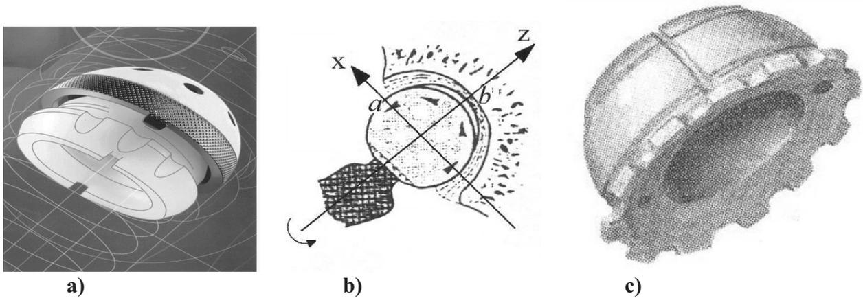
Fig. 4. Elliptical friction nod: a) complete elliptical prosthesis of human hip joint, b) elliptical bone head, c) the elliptical sleeve in the humanoid robot bearing
