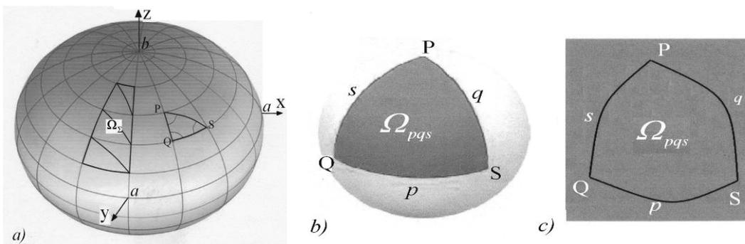
Fig. 6. Elliptical triangles: a) Lubrication region  $\Omega_{\Sigma}$  lying on the elliptical slide bearing surface as a sum of elliptical triangles with the vertexes  $P, Q, S$ ; b) Enlargements of elliptical triangle  $PQS$  on the elliptical surface; c) elliptical triangle on the plane
