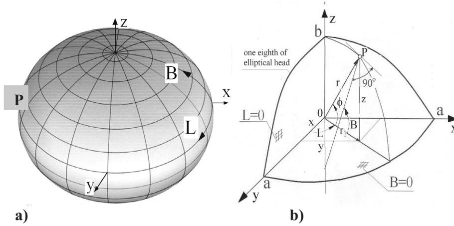
Fig. 5. Coordinates for the arbitrary point lying on the elliptical head surface: a) wide coordinate  $B$  and length coordinate  $L$ , b) connexion between Cartesian coordinates  $(x, y, z)$  of arbitrary point  $P$  lying on the elliptical surface and its wide  $B$  and length  $L$  coordinates
