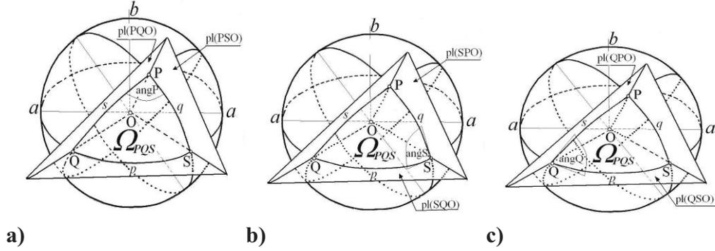
Fig. 7. Elliptical triangle surface  $\Omega_{pqs}$  and planes  $pl(PQO)$ ,  $pl(PSO)$ ,  $pl(QSO)$  to be created by the three points  $P, Q, O$ , and  $P, S, O$  and  $Q, S, O$  respectively, where  $O$  is the centre of ellipsoid
