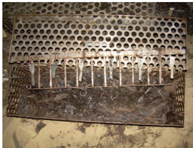
FIGURE 3. THE BASKET WITH TESTED SAMPLES AND COMPOST
