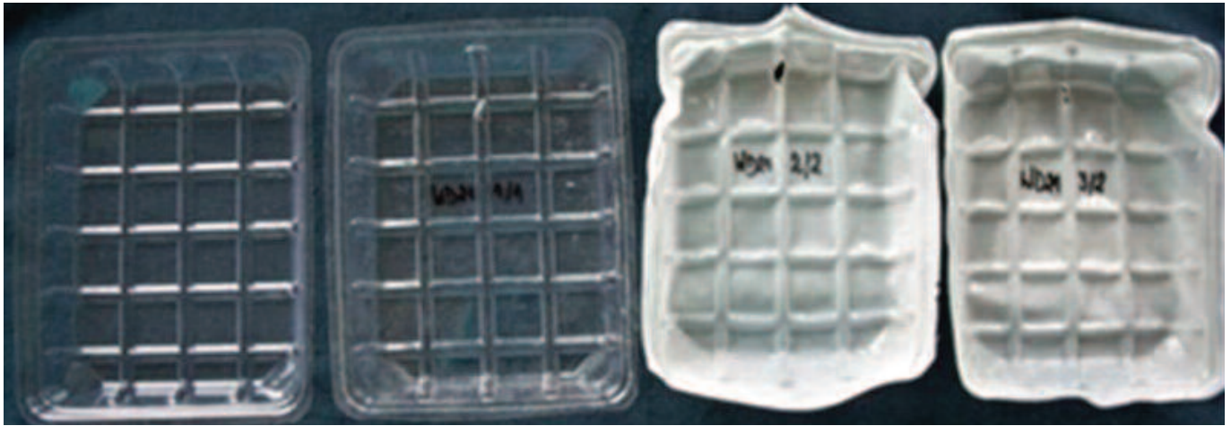
FIGURE 4. DIGITAL PHOTOGRAPHS OF THE THERMOFORMED FINAL PRODUCT FROM PLA RIGID FILM BEFORE AND AFTER 1, 2 AND 3 WEEKS OF DEGRADATION IN A KNEER SYSTEM CONTAINER
