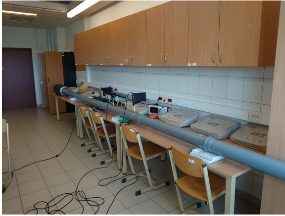
Figure 1. The experimental waveguide. The left side of the photo shows the speaker enclosure.
