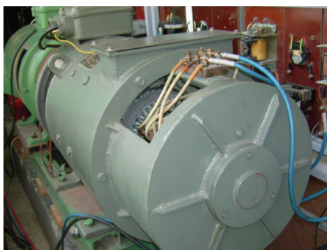
Fig. 1. Separately excited DC motor
