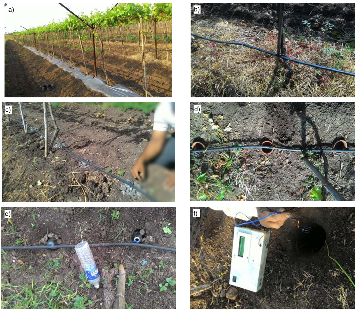
Photo 1. Photographic views of experimental work on the field: a) drip irrigation with plastic mulching (DIPM), b) drip irrigation with organic mulching (DIOM); c) subsurface irrigation stone column (SISC), d) subsurface irrigation with mud pot (SIMP), e) subsurface irrigation with plastic bottles (SIPB), f) moisture sensor and its recording device (photo: S.J. Kadhbane)
