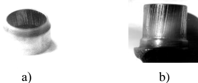
Fig. 4. The appearance of worn parts («false brining») of the bearing assembly of the crosspiece a) – the bearing cage; b) – the axle of the crosspiece
