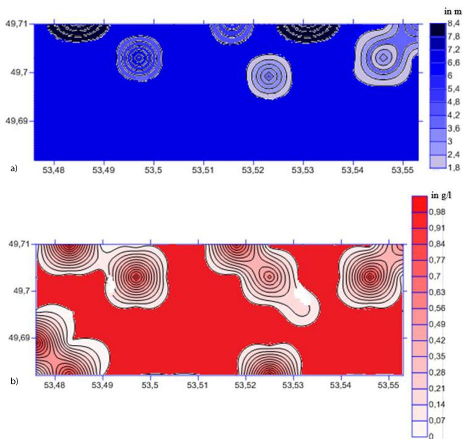
Figure 5. Isolinear map of GWL (A, m) and GWM (B, g/l) of the Alymshagyl sand massif
