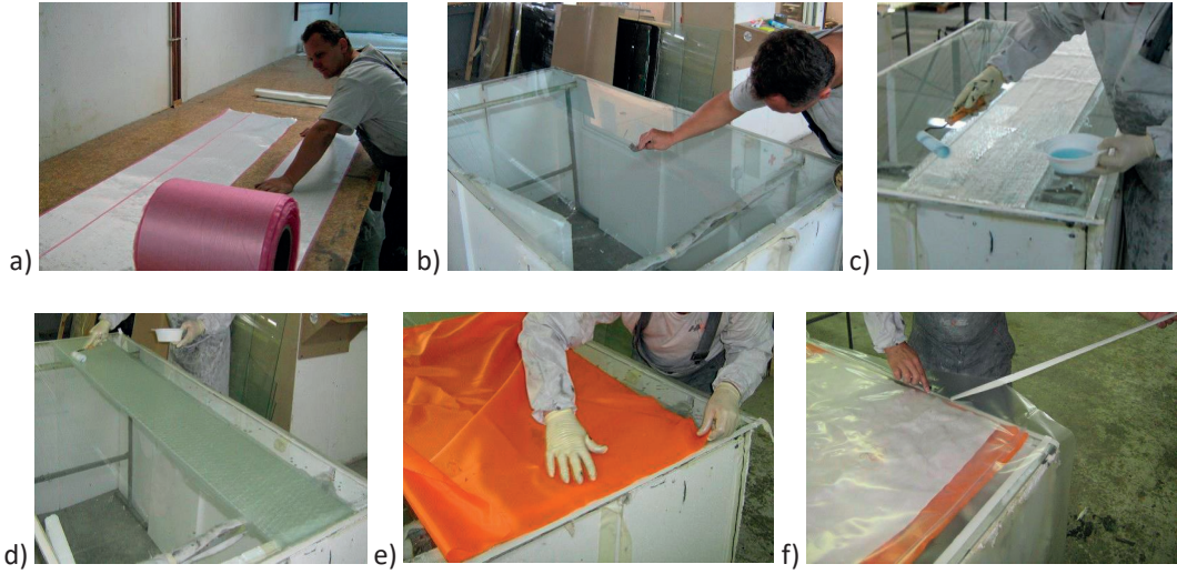
Fig. 1. Forming stages of the composite material II made by vacuum bagging: a – cutting out and preparing the reinforcement; b – mold surface preparation; c – soaking individual laminated reinforcement layers with resin; d – ready composite material II; e – application of auxiliary layers under the film, such as peel ply, breathing material; f – application of a double-sided sealing tape made of special bonded film around the edge of the mold, under which the components of the composite material (and auxiliary material) had been present [Chatys, 2015]
