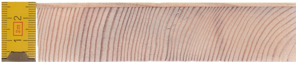
Fig. 6. Cross section of a two-layer (ash/pine) floor element.=
