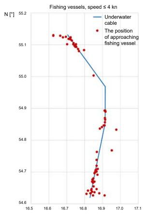
Figure 8. Closest position of fishing vessels to the underwater cable (distance less than 3 Nm, speed less than 4 knots)
