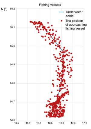
Figure 7. Closing fishing boats situations to underwater cable independently boat speed. VMS data
