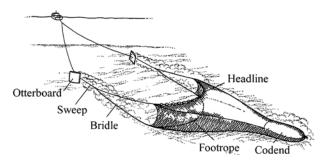
Figure 2. Schematic diagram of an otter trawl (Palanques, Guillen & Puig, 2001)
