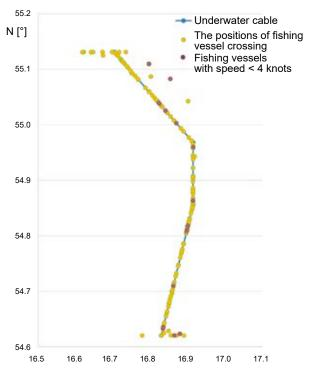
Figure 9. Positions of fishing vessels passing over the underwater cable from the AIS data
