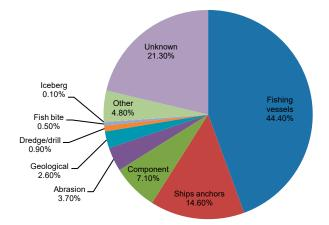
Figure 1. Underwater cables damage statistics. Data collected by the Department of the Interior, Bureau of Ocean Energy Management, 2014
