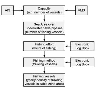
Figure 5. Scheme for estimating which trawling fishing vessels are a danger to underwater cables
