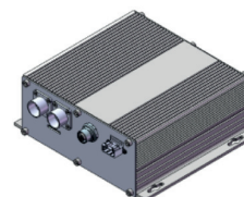
Fig. 7. Visualization of the chassis the Internet and Intranet access module (LTE Router) [own study]
