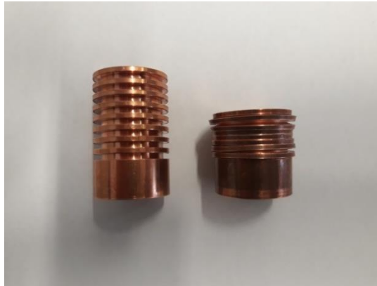
Photo 7. Copper fenders. On the left – fender before the G-force test, on the right – fender after the G-force test. As a result of the impact, the fender was shortened by 13 mm
