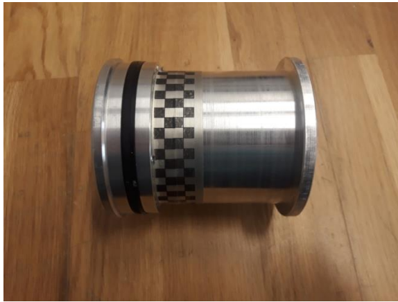
Photo 5. Projectile with the installed telemetry module of the cal. 155 mm guided ammunition, prepared for acceleration tests
