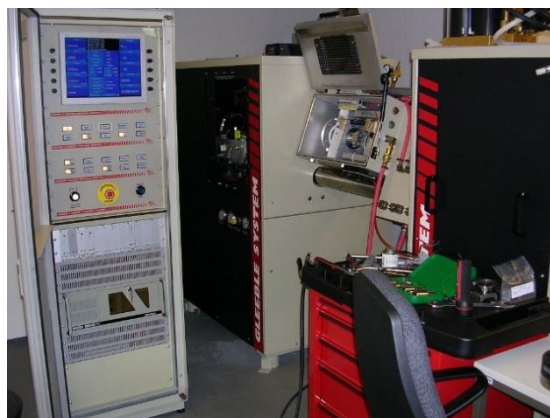
Fig. 4. Gleeble 3800 thermo-mechanical simulator
