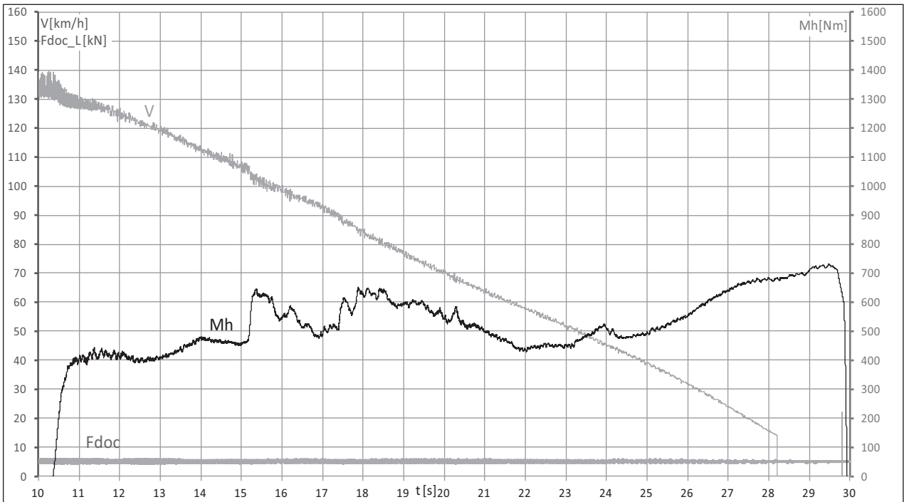
Fig. 7. Test 221, ABS-off, non-slippery surface, pushing force 5 kN
