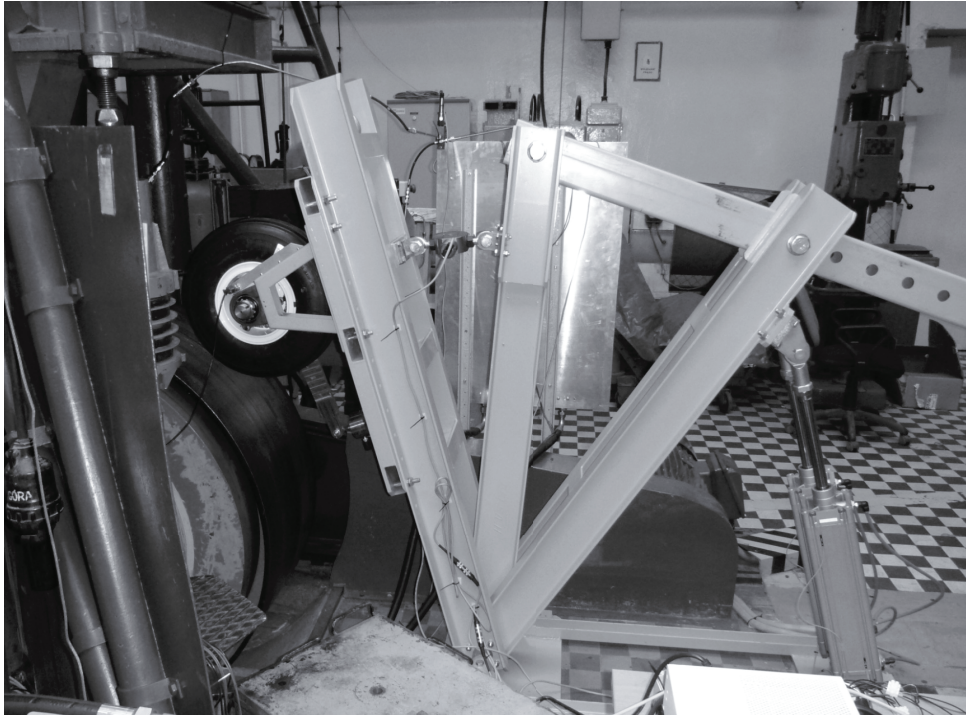
Fig. 6. M3T test stand adds on for ABS system tests (source: IoA)
