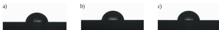
Fig. 9. Images of water drop on the surface of: a) LDPE, b) LDPE + 1 wt% \text{TiO}_2\text{-SiO}_2 , c) LDPE + 1 wt% \text{TiO}_2\text{-SiO}_2/\text{POSS}
