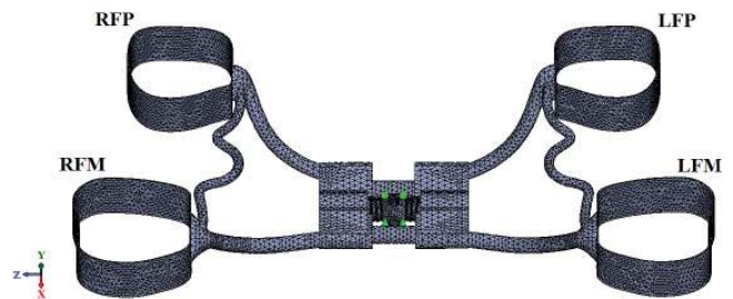
Fig. 1. Model of the midpalatal expansion device with Hyrax screw – finite element mesh used in simulation
